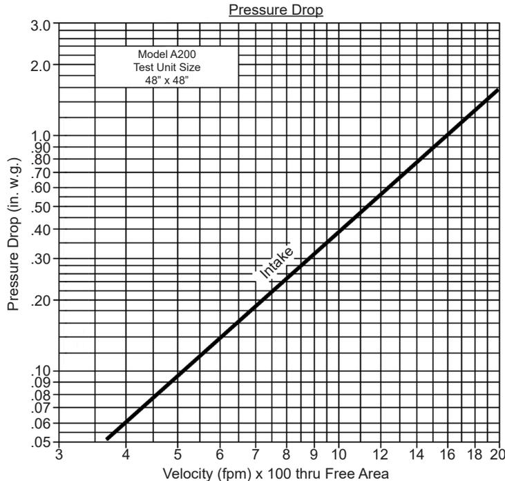
Intake air converted to standard air density.
